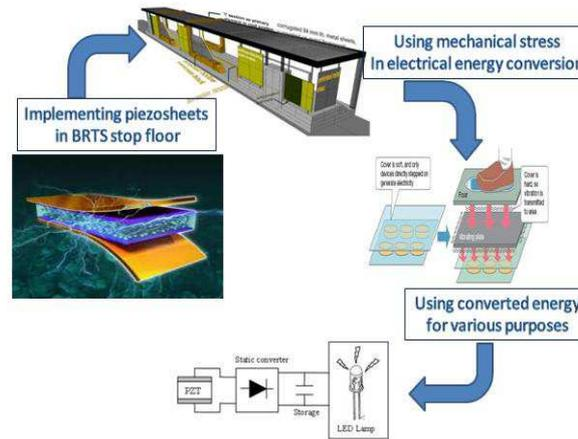
**Figure 3: The Implementation of Piezosheets and Utilization of Power Generated**
