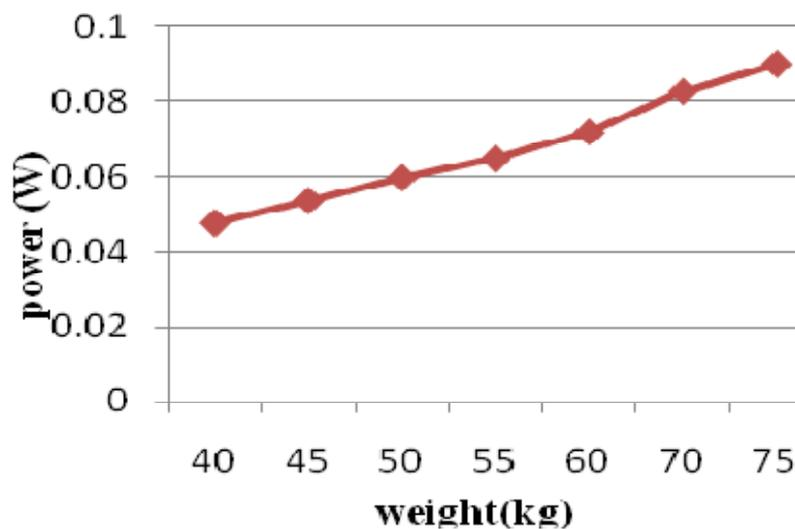
**Figure 4: Graph between Weight Applied & Power Generated by Piezosheets**
