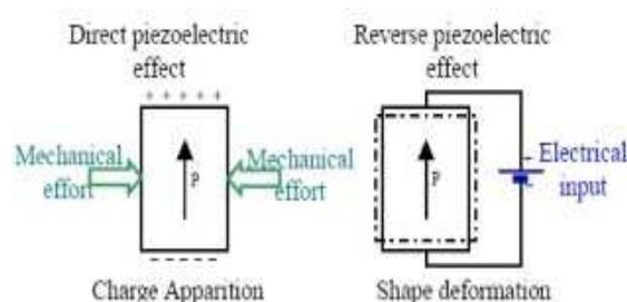
**Figure 2: The Process of Electrical Energy Production by Piezo-Crystals**
